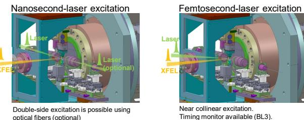
Double-side excitation is possible using optical fibers (optional)
