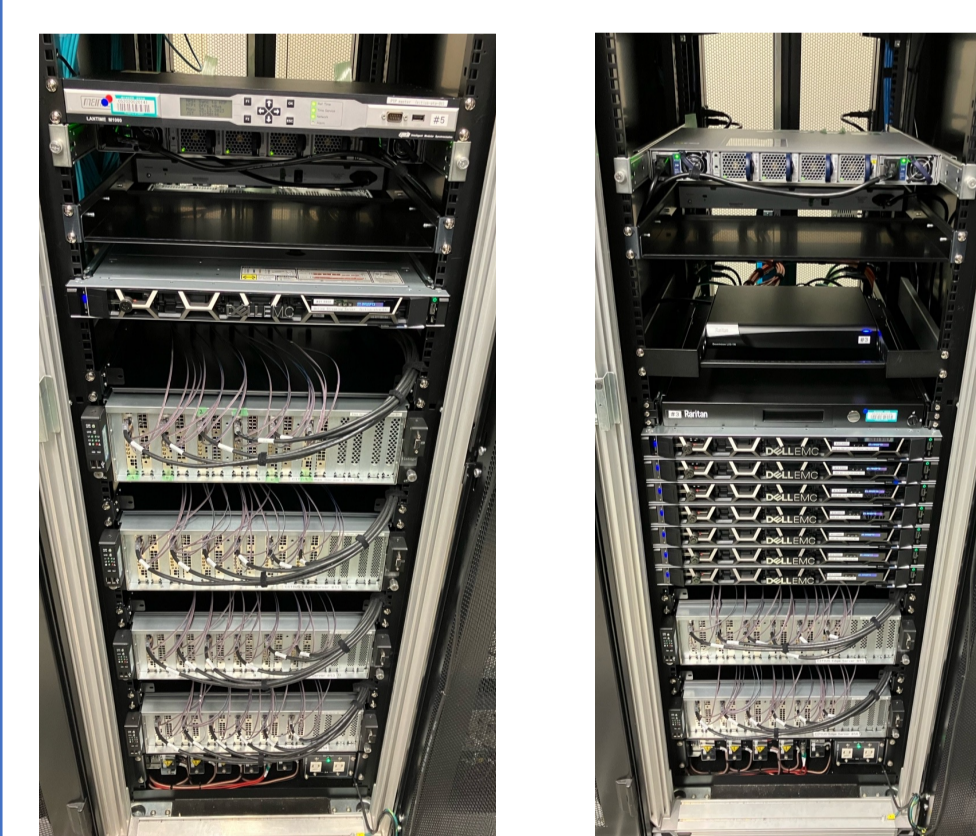
Data acquisition computers for CITIUS-20.2M installed in the server room of SACLA
